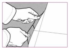
When the width of the room exceeds the sheet width (more than one piece has to be installed to cover the area), mark a line on the floor parallel to the longitudinal wall at a distance equivalent to 12 cm (about 41/2 in.) less than the sheet width. Mark the room's center on this line. On the bottom of each sheet, mark their center. The cross marks on the subfloor and sheets shall coincide at installation.
