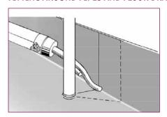
Around pipes by walls, cut the sheet and press it against the pipe to form a collar. In tight or cramped areas between pipes and walls, cut as shown by the dotted line. If a cover is required, do the following:
