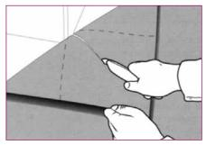
When fitting an out-corner, the sheet is folded against the corner and cut about 5 mm( ¼ in.) from the floor. The guidelines in the picture show the corner on the sheet and the position of the cut at about a 45- degree angle. Then a diagonal cut is made as shown.
