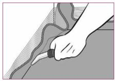
Use a Tarkett Hockey Stick or Tarkett Corner Roller to press the material firmly into the juncture between the floor and wall. In areas where one sheet is sufficient to cover the subfloor, the adhesive can be applied over the entire surface area before installing the sheet. Although this requires experience, it is the fastest installation method.
