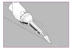
Weld with hot-air and Tarkett Speed Welding Nozzle. Carry out a test welding on a leftover piece before commencing work, to adjust speed and temperature
