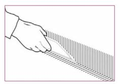
Using a straight edge and pencil, mark at a height of about 10 cm (approx. 4 in.) all walls where the flooring will be coved. Apply the adhesive on the walls up to the marked line, using a finenotched trowel.
