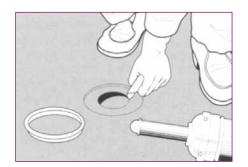
Around flush drain openings, heat the sheet and mark the location of the drain using a clamp ring. Then cut a small hole in the centre of the drain within the mark. Heat the flooring and press the clamp ring down into the edge of the drain. When using an adjustable clamp ring, make sure it fits tightly. Trim the material around the perimeter of the ring.
