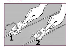
CAUTION: Welded seams must cool to room temperature before trimming. Start trimming where you began welding. All trimming of welding thread is recommended in two steps: rough and fine trimming.
