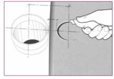
Around drain pipes, fold the sheet against the pipe and mark a line on the material where the center if the pipe is. Cut a hole about 25 mm (about 1 in.) smaller than the diameter of the pipe. As shown, cut the hole at the start of the fold. Heat the sheet vinyl and press it over the pipe. trim off excess material with o hook knife so that the break in the pipe wall is cleared.
