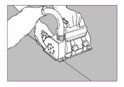
The sheets are heat welded. Do not weld until the adhesive has bonded completely. The joints are chamfered or grooved to about ¾ of the thickness using a hand grooving tool or machine prior to welding.
